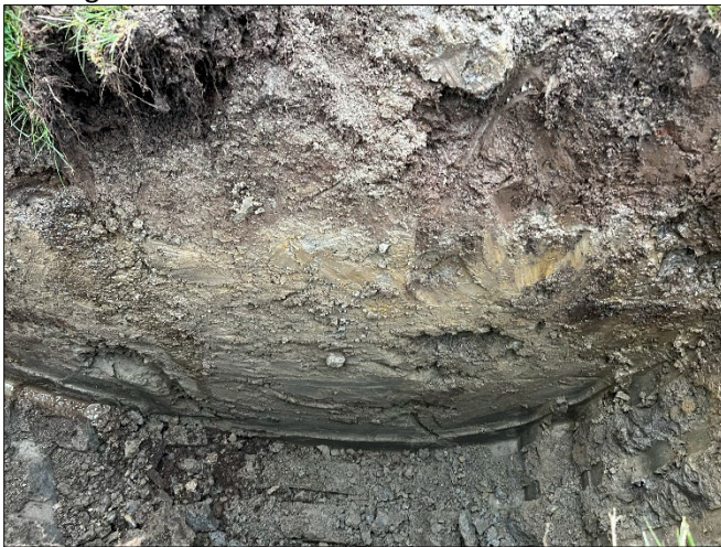
Photo 3: TP-1 conditions. Note mottled GMD layer overlying very stiff/hard glacial drift.
